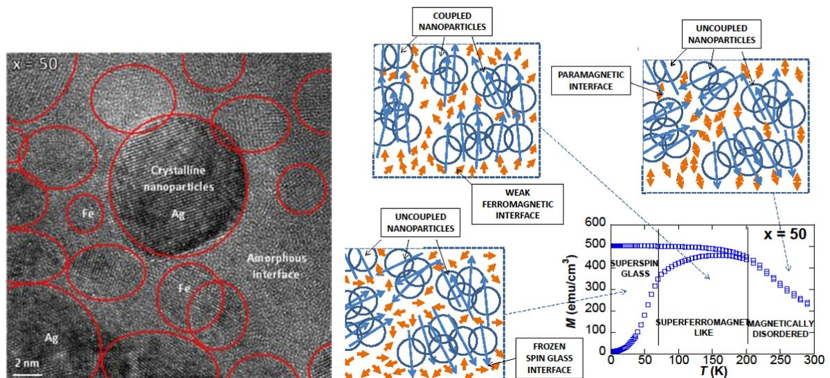
FIG1: (left) High resolution transmission electron micrograph obtained for a  $Fe_{50}Ag_{50}$  sample deposited by PLD. Ellipsoids mark the positions of some crystalline nanoparticles. (right) Picture of the thermal evolution of the magnetic structure for a  $Fe_{50}Ag_{50}$  thin film. Simplified pictures of the magnetic moments configurations in three ranges of temperatures are also included.
